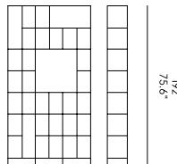
**EN** — Painted metal bookcase. Removable thermoformed shelves in eco-leather, equipped with magnet for locking on the structure of the bookcase. Two or more modules can be combined and joined by means of a clip supplied in the assembly kit. Adjustable feet.
